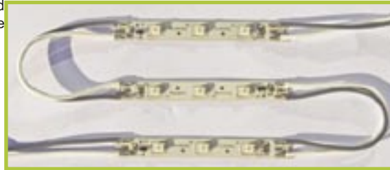
∞^ Approximately 3.5 to 4 inches of flexible wiring connects the Light Strips.
